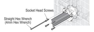
(6) Then, use L-shaped 4mm Hex wrench to fully tighten and fasten it.
